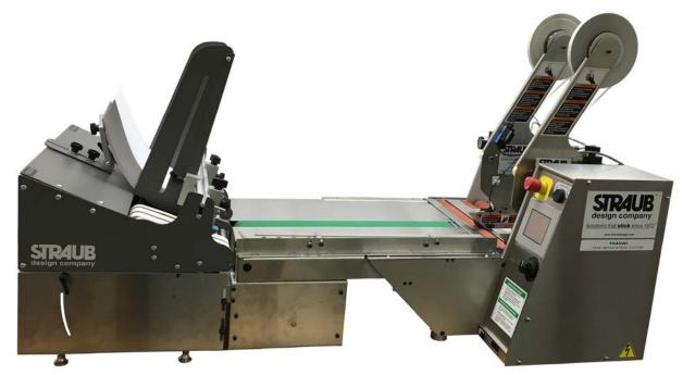
The T-646 Tape Application System is a bench-top system that applies strips and/or spots of many types of adhesive transfer, double coated and foam tapes to flat surfaces. These systems are available with many different options. See the individual Data Sheets for additional information. Shown is an SF-20 Feeder with an AS-20 Alignment Section and a T-646I Base Unit with two T-646WH Applicators.
