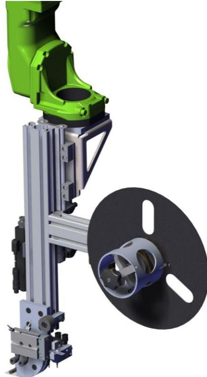
RH VERSION WITH KNICK & BREAK KNIFE ASSEMBLY SHOWN
