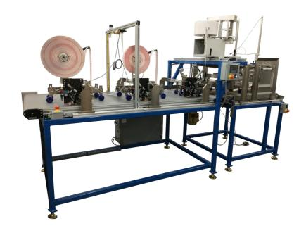
and the product. The product is then conveyed out of the machine for additional processing. Top loading of feeder permits loading while machine is operating.
