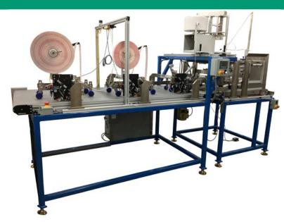
depending on the tape and the product. The product is then conveyed out of the machine for additional processing. Top loading of feeder permits loading while machine is operating.
