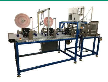
The automatic feeder feeds the blanks to a conveyor where one or more tapes are applied automatically using T-626 tape applicators at up to 350' per minute. The product is then conveyed out of the machine for manual processing.
